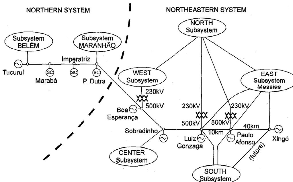
Figure 1 - Simplified one-line diagram of Brazilian Northern-Northeastern system
